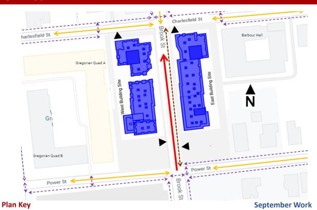
2 Way Vehicle Traffic Pedestrian Traffic Construction Site Access
